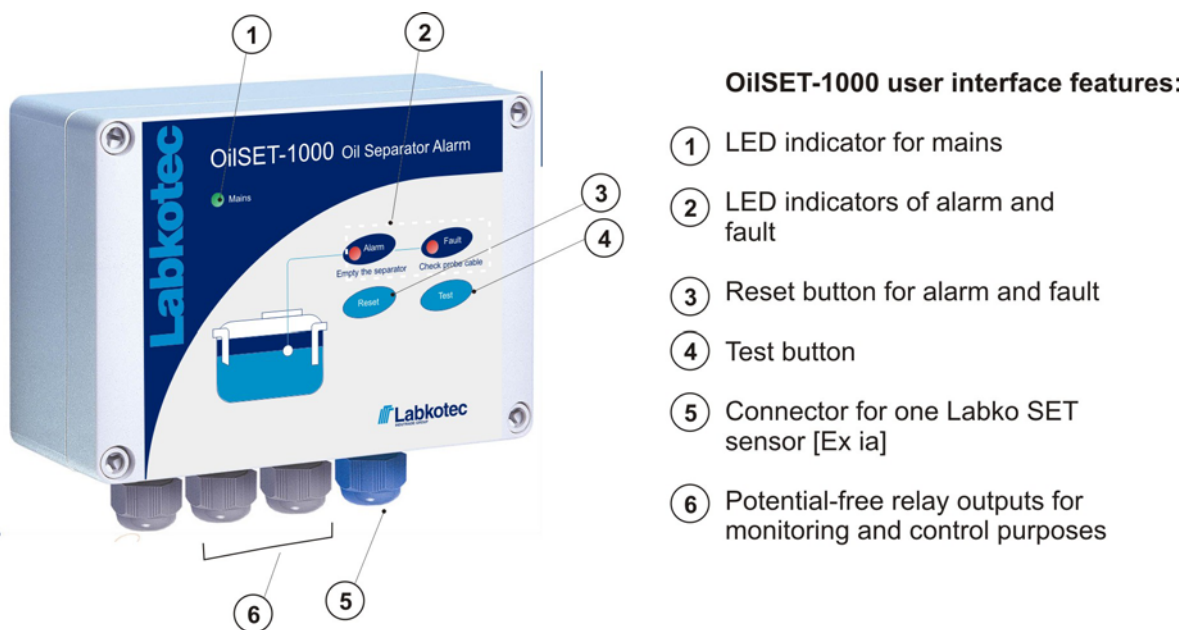
Figure 2. OilSET-1000 control unit - features
